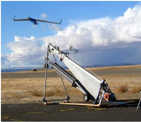
Figure 3. The ScanEagle is launched from a catapult (the image is from http://www.insitugroup.com/pages/Product/s/seascanSpecs.html )
